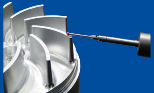
DEA GLOBAL PERFORMANCE 9128 Coordinate Measuring Machine (CMM) fitted with a TESASTAR-M head, and a LEITZ LSP-X1 continuous scanning probe
