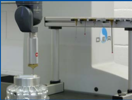
DEA GLOBAL PERFORMANCE 9128 Coordinate Measuring Machine (CMM) fitted with a TESASTAR-M head, and a LEITZ LSP-X1 continuous scanning probe
