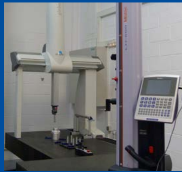
DEA GLOBAL PERFORMANCE 9128 Coordinate Measuring Machine (CMM) fitted with a TESASTAR-M head, and a LEITZ LSP-X1 continuous scanning probe
